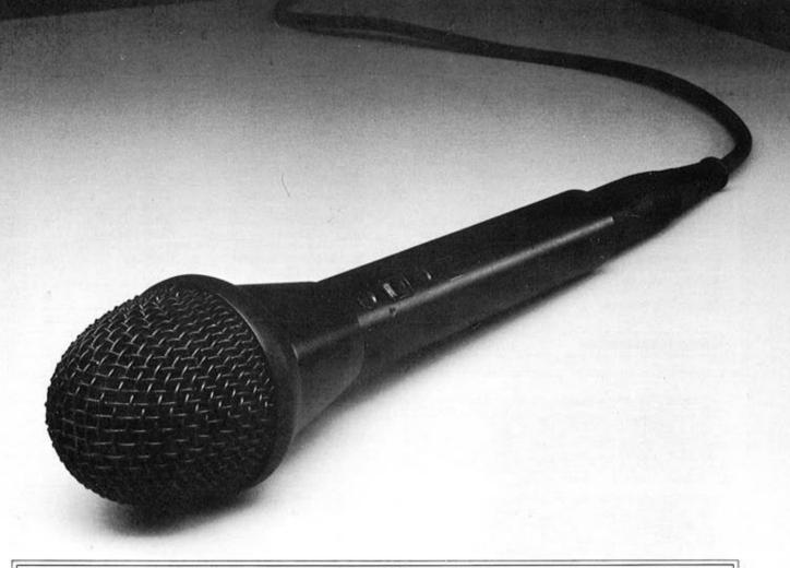
Features: he BM-73 is a versatile cardioid condenser microphone for operation on 48 volt MIPOW® system. The circular condenser element is mechanically insolated from the case by a built in elastic shock resistant suspension, and an electronic proximity filter is designed into the microphone. This is to reduce unwanted noise as well as
