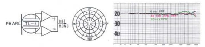
If the signals from membranes I and II are added equally to one mono signal, the recording characteristics become high quality omnidirectional.
